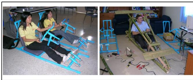
Figure 6. Racing game controllers made from PVC water-pipe (left) and bamboo (right).
